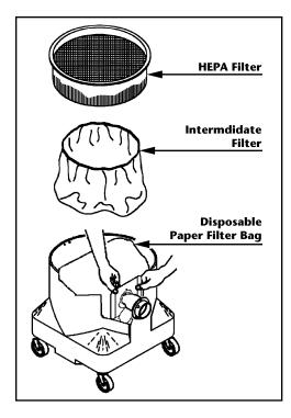
This hazardous waste vacuum has special filters installed. The disposable paper bag filter contains the bulk of all debris and protects remaining filters from excess dirt. The intermediate filter is a very fine nonwoven filter that extends the life of the expensive High-Efficiency Particulate Air (HEPA) filter.
